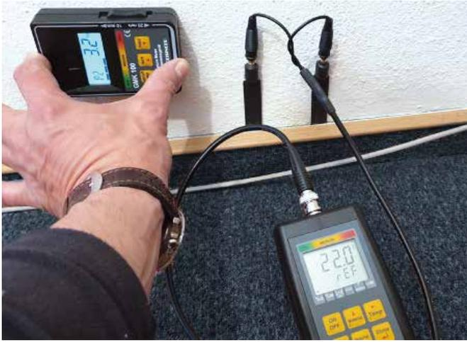
Measurement in screed insulation through edge insulation strips:
