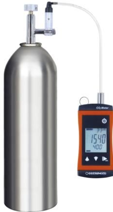
Calibration with test gas GZ-18 and adapter GZ-19
