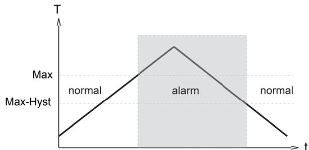
A changeover delay time ( $t_{DS}$ ) can be applied to switching to the alarm state. One switch-back delay time ( $t_{DR}$ ) of several can likewise be applied to switching back to the normal state.
